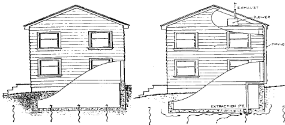
Figure 1 - Schematic Diagram of Typical Residential SSD System
